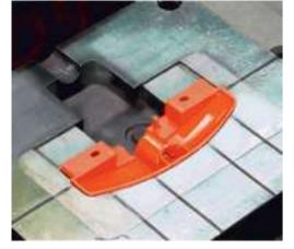
Injection mould - Impact 200 end piece
