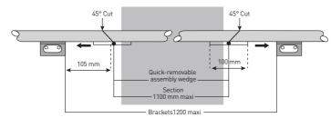
For Escort handrail, Rapid'Access<sup>®</sup>, the articulated link has been especially designed for service duct, to complete with one quick-removable assembly wedge. (available in chalk or anodised look)
